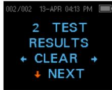
3. Press the LEFT or RIGHT control panel button to clear the results.
