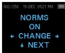
The NORMS setting allows you to display the Expanded Boys Town Norms template on the value graph for eligible DPOAE protocols. The normative data does not affect the *Pass/Refer* criteria or the results of the DP screening test. Norms are for viewing purposes only.<sup>1</sup>
