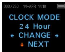
3. Press either the LEFT or RIGHT control panel button to change from the 12- to the 24-hour mode or from the 24- to the 12-hour mode.
