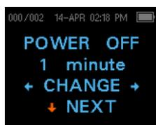
3. Press either the LEFT or RIGHT control panel button to change to the desired interval.
